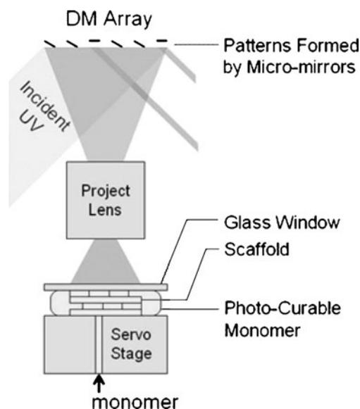
**Fig. 1** Illustration of the DMD-PP apparatus for developing 3-D scaffolds with heterogeneous material properties
