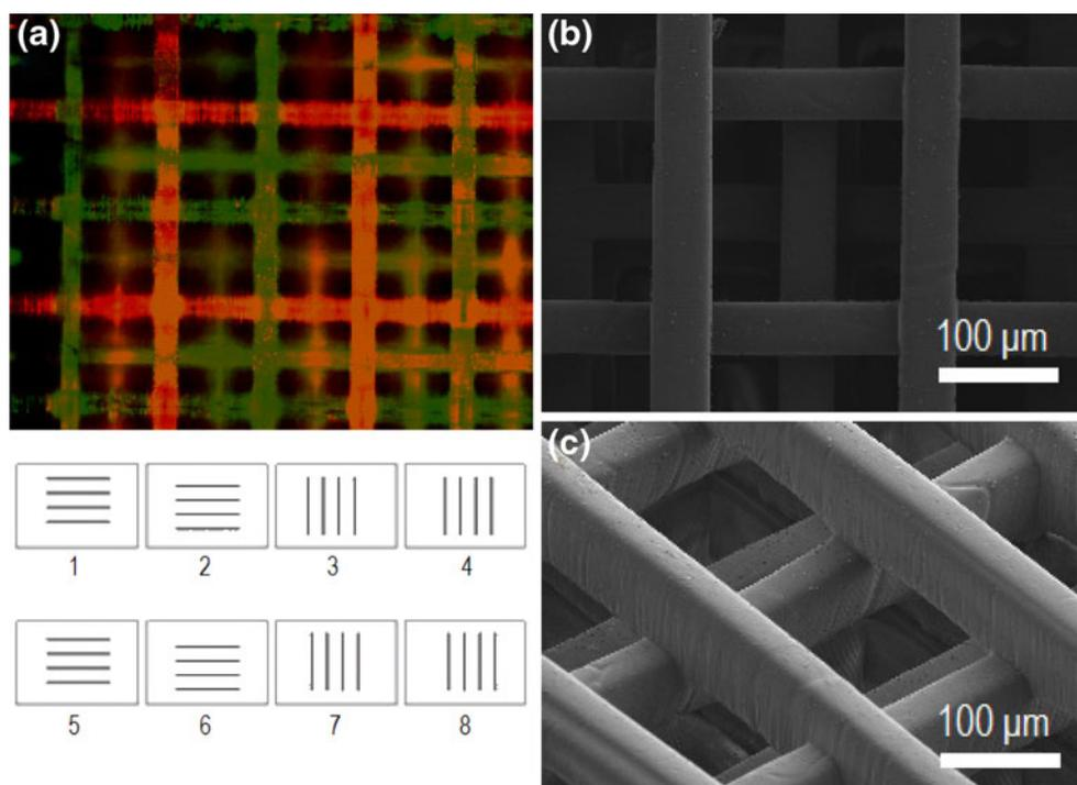
UV-exposure, solvent purging, and monomer switching processes were repeated until the entire scaffold was fabricated.
