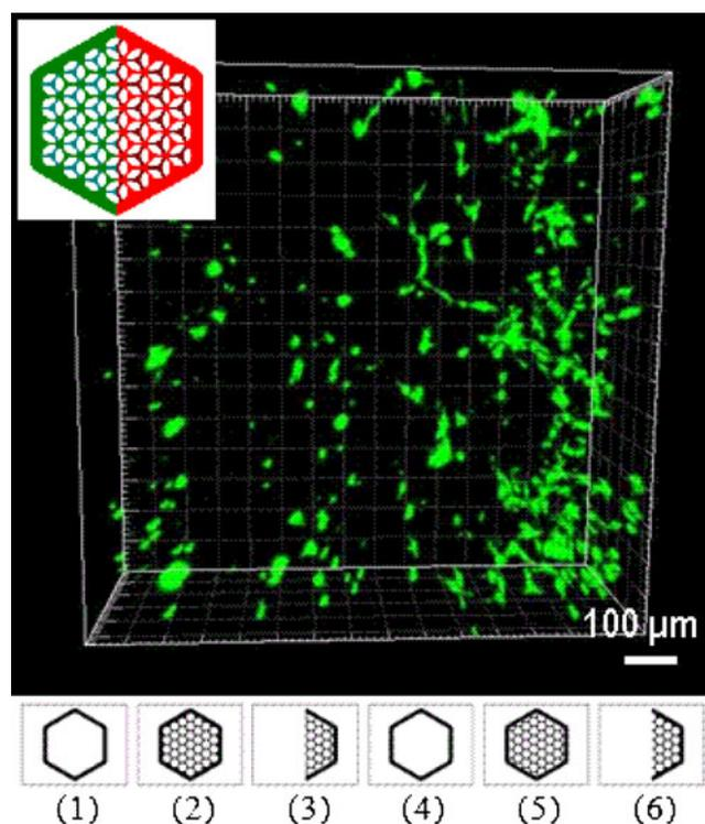
**Fig. 4** The fabricated honeycomb microstructure is composed of cell-adhesion sites (pattern 3, 6) and blank structures (pattern 1, 2, 4, 5). Cell aggregation and adhesion are observed in the half of the scaffold where protein was conjugated
